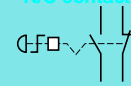
Emergency stop trigger action mushroom head Turn to release N/O + N/C contact
