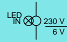
Pilot light with integral transformer, 230 V c primary, 6 V secondary. BA 9s incandescent bulb or LED
